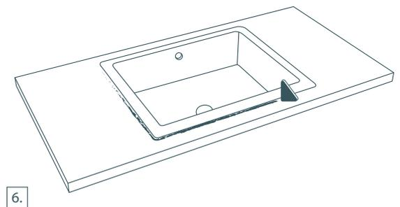
Topmount washbasins are suitable for all countertops and they are easily mounted in a standard way.
